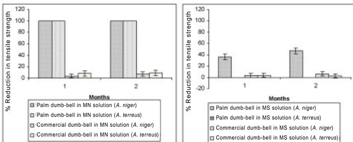
Figure 12. Reduction in tensile strength (%) of palm-based and commercial foams in MN (left) and MS (right) solution in shake flask test.
