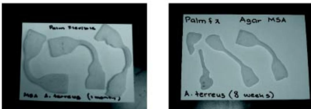
Figure 4. Palm-based foams incubated in MS solution in shake flask test after one (left) and two months (right).
