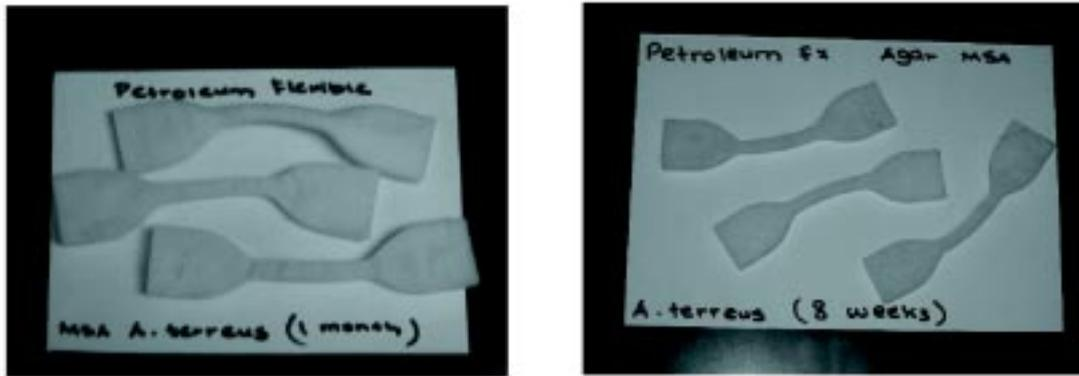
Figure 5. Commercial foams incubated in MS solution in shake flask test after one (left) and two months (right).
