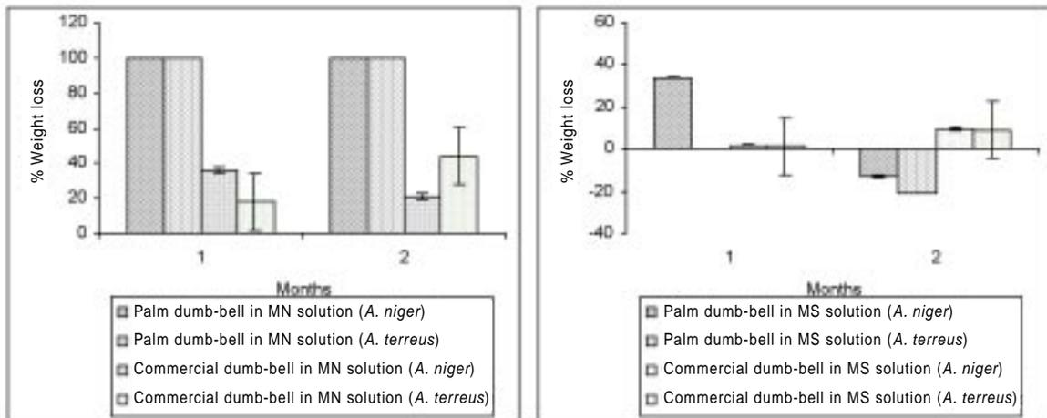
Figure 9. Weight losses (%) of palm-based and commercial foams in MN (left) and MS (right) solution in shake flask test.
