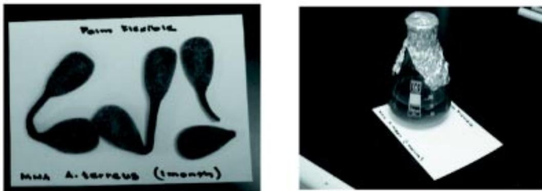
Figure 2. Palm-based foams incubated in MN solution in shake flask test after one (left) and two months (right).
