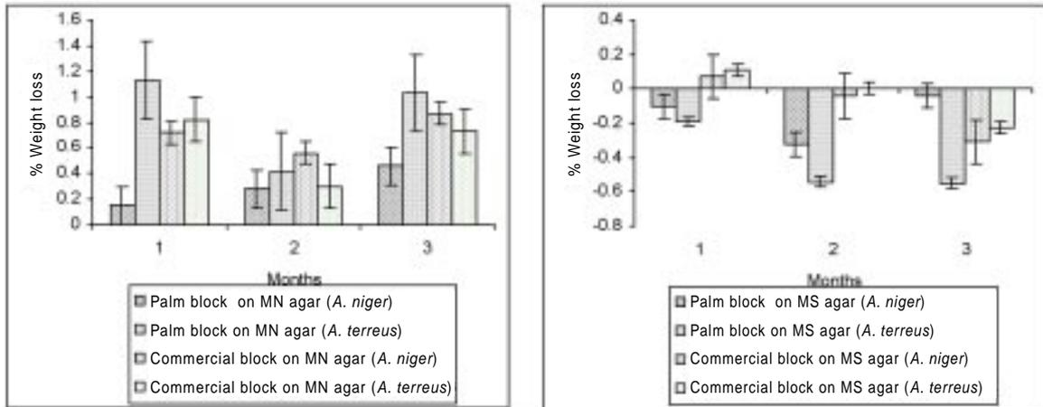
Figure 8. Weight losses (%) of palm-based and commercial foams incubated on MN (left) and MS (right) agar in petri dish test.
