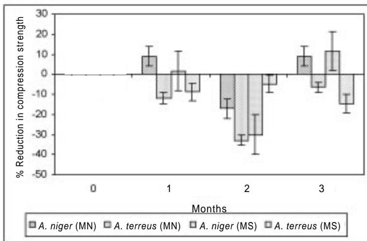
Figure 10. Reduction in compression strength (%) of palm-based foams in petri dish.
