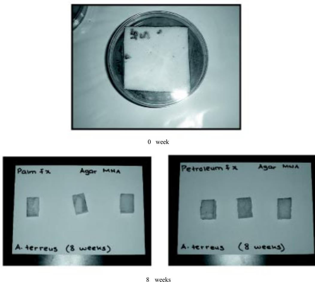
Figure 1. Growth of *A. niger* and *A. terreus* on palm-based flexible foam (left) and commercial foam (right) at 0 and 8 weeks' incubation on MN agar in petri dish test.
