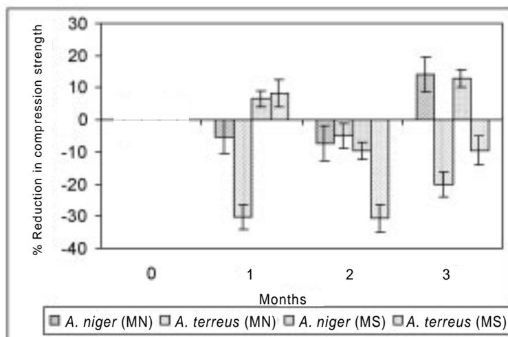
Figure 11. Reduction in compression strength (%) of commercial foams in petri dish test.
